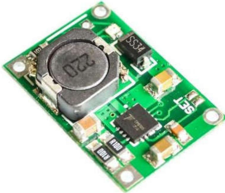
TP5100 is a double switch buck 8.4V, single cell 4.2V lithium battery charge management chip. Its ultra-compact QFN16 package and simple external circuit, making TP5100 ideal for portable equipment so large current charging management applications. Meanwhile, TP5100 built-in input overcurrent, undervoltage protection, over temperature protection, short circuit protection, battery temperature monitoring, reverse battery protection.
